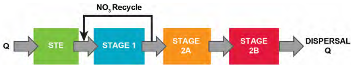
Figure 15. Example Flow Diagram: In-Tank Two Stage Biofilter with Recirculation Stage 1, Dual Media Stage 2 Lignocellulosic (2a) Followed by Elemental Sulfur (2b) (Hazen and Sawyer 2015b)
