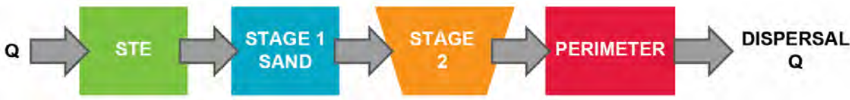
Figure 16. Example Flow Diagram: In-Ground Stacked Biofilter, Single Pass Stage 1 Over Stage 2 Lignocellulosic (Hazen and Sawyer 2015b)
