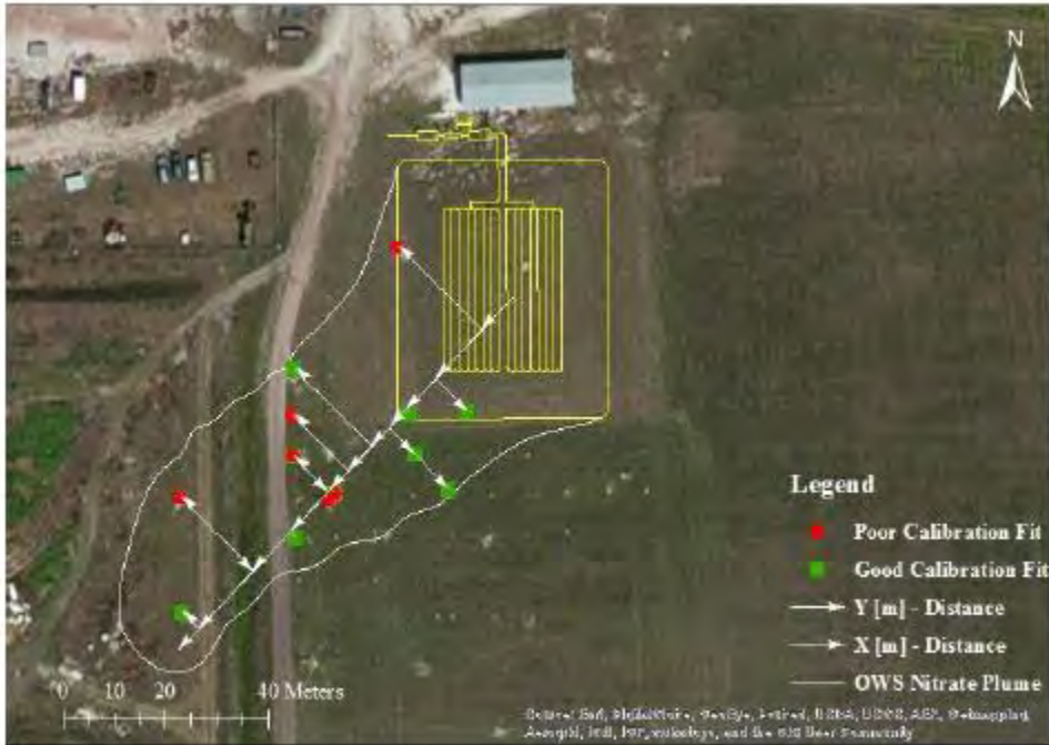
Figure G- 7. Method Used to Estimate X, Y, and Z Values Required by the Aquifer Model to Calculate Concentration (Hazen and Sawyer 2015c)
