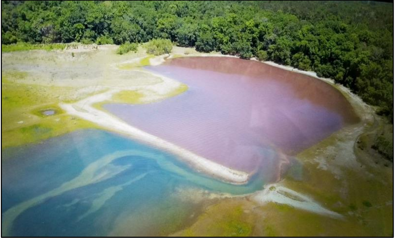
Figure 4.20. Dye backup into Upper Lake Lafayette after draining of Buck Lake, April 17, 2018.
