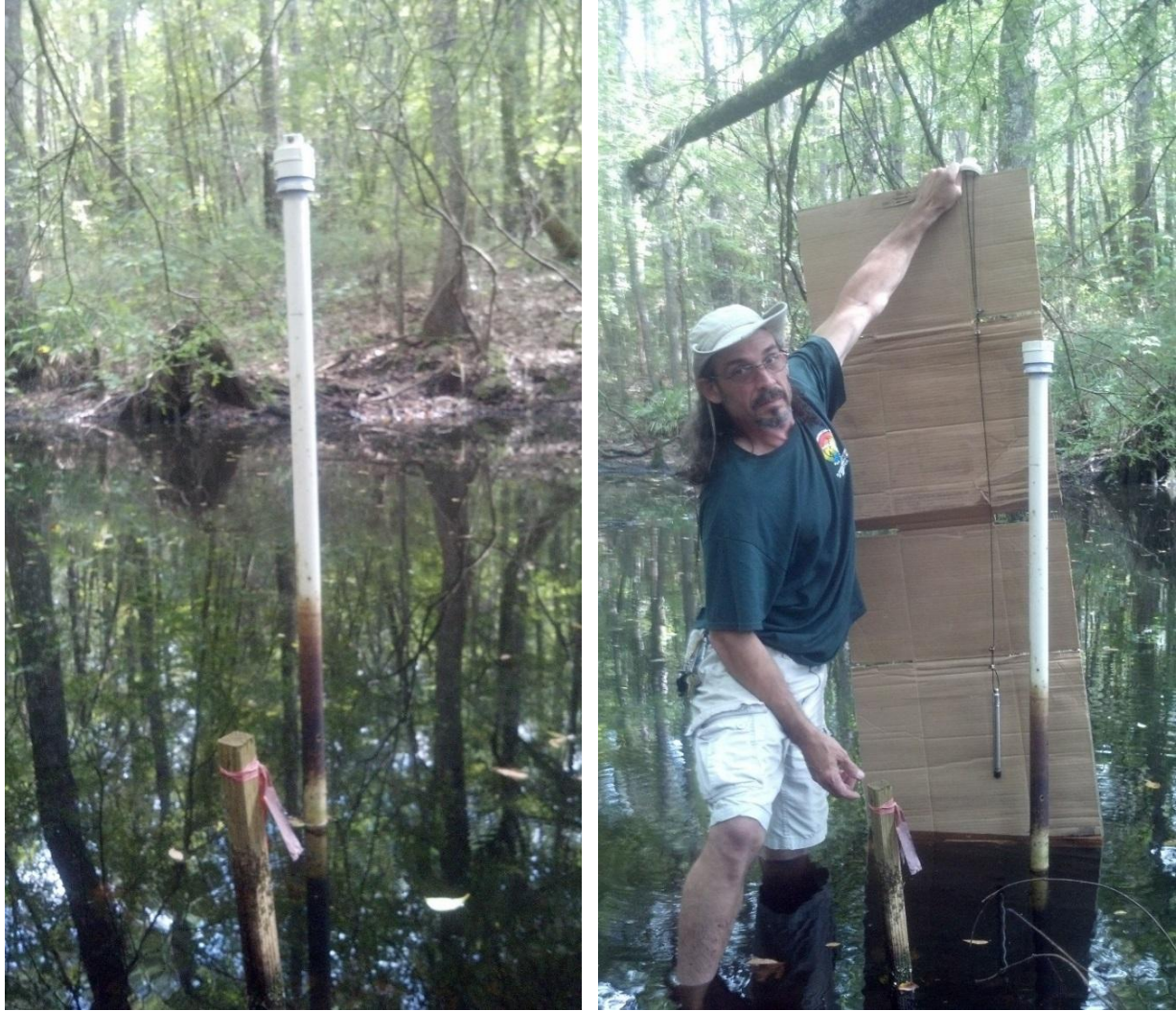
Figure 4.4: Revell Sink water level elevation station; left view, level logger in deployed mode; right view, level logger removed for perspective of top of casing, depth of deployment, and transducer elevation.
