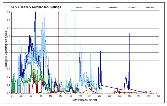
Uranine Dye (AY73) recovery curves for Indian Spring (IS), Sally Ward Spring (SWS), Wakulla B-Tunnel (WKB), Wakulla Vent (WKV), and McBride's Slough (MBE) resulting from dye injections performed at the City of Tallahassee's waste water spray field.
