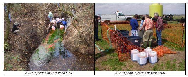
Photos of the dye injections that occurred at a swallet and monitoring wells located within the City of Tallahassee's waste water spray field.
