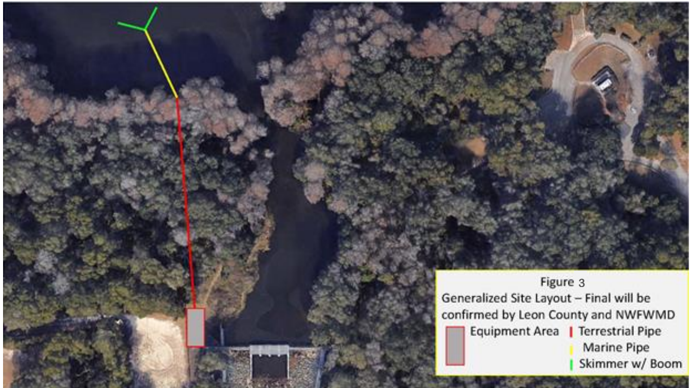
Figure 3. Conceptual Site Layout. Final site layout will be in conformance with to-be-issued Leon County Temporary Uses, Construction Staging Areas and Special Events Permit.
