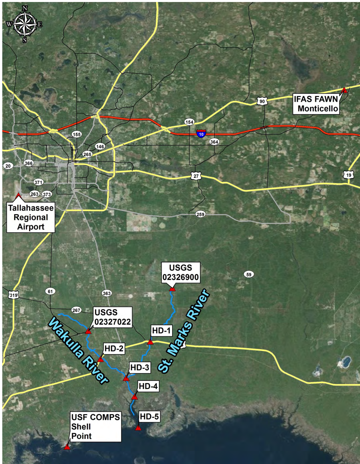
Figure 5. Locations of data collection sites for continuous recorders (HD-1 through HD-5), USGS flow gages, USF COMPS Shell Point winds, Tallahassee Regional Airport meteorology (including rainfall), and IFAS FAWN Monticello.
