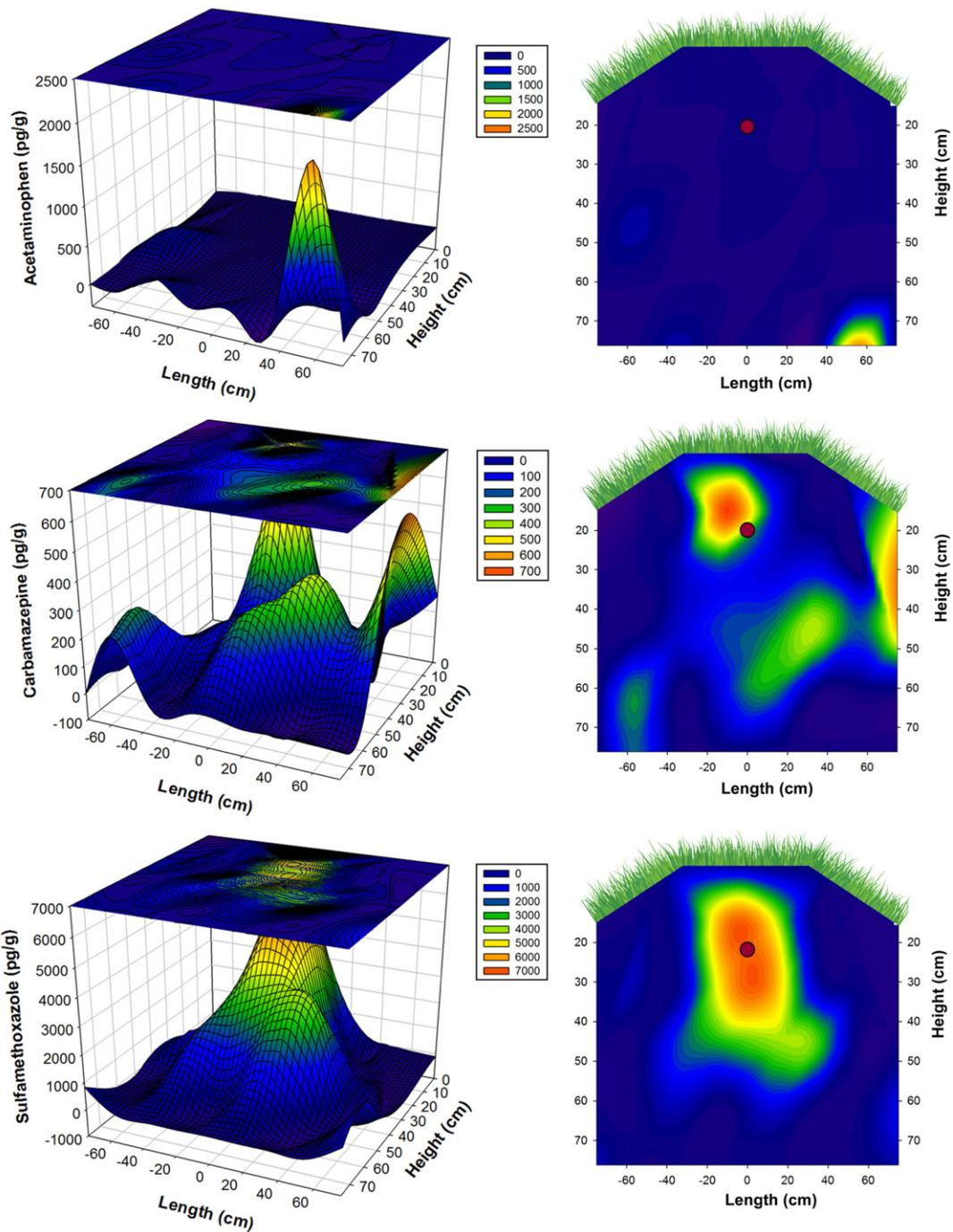
**Fig. 2.** Spatial distribution of micropollutants within septic system drainfields (36 locations). Drip pipe was installed at a height of 22 cm from the top (red dot). Negative numbers on x axis represent the left side of drainfield.
